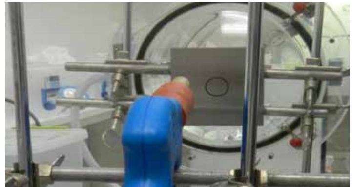
Inoculated plates mounted for exposure and steam cleaned for defined exposure times
